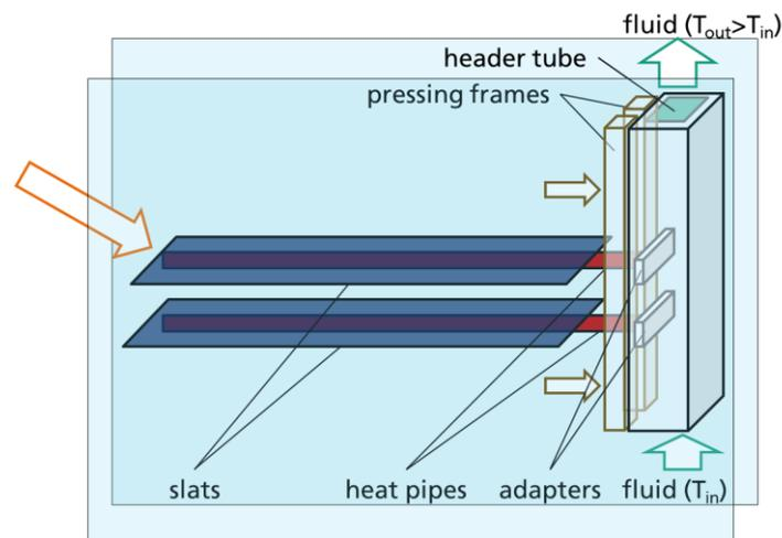
Figure 1: Working principle of solar thermal venetian blind
