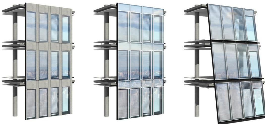
Figure 2: Visualization of three different façades with STVB, variety *low g-value*
