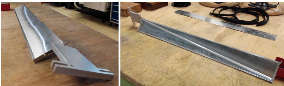
Figure 4: First produced slat of proof-of-concept test sample with adapter visible in the foreground (left) and bottom view with diagonal heat pipe mounting (right)
